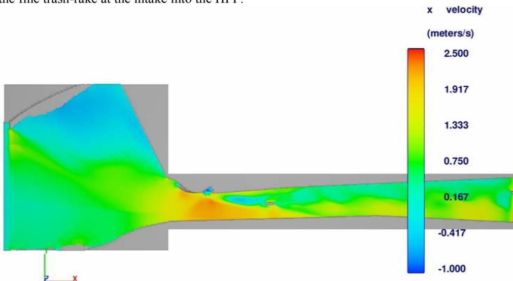
Fig.9. Modification of the left wing wall of the intake without the pier at the flow  $Q_{S1+S2} = 24 \text{ m}^3/\text{s}$
