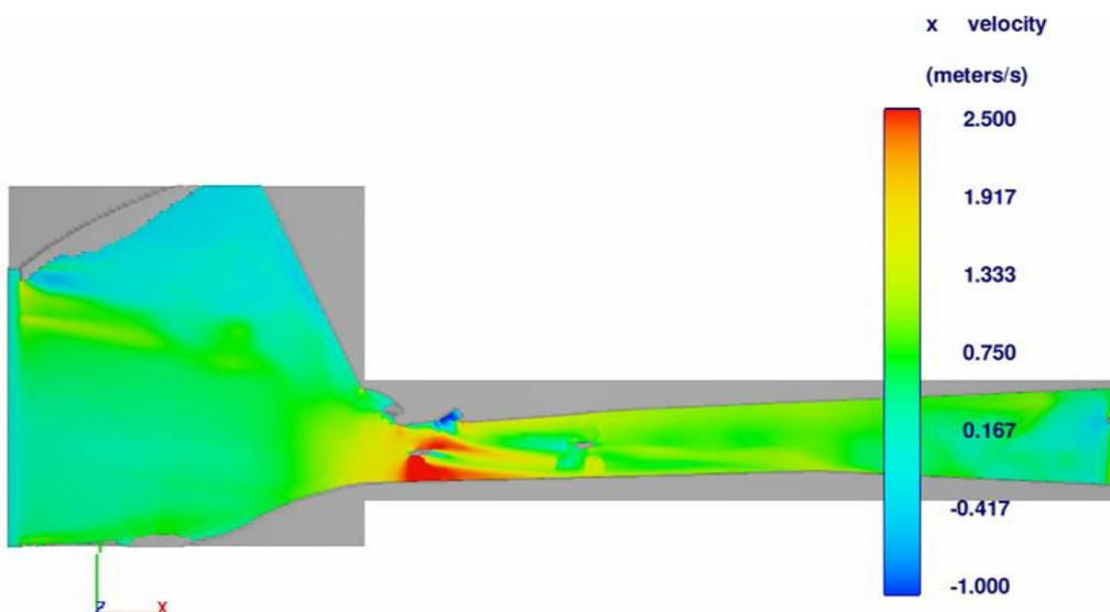
Fig. 6. Existing condition at the flow  $Q_{S2} = 18.3 \text{ m}^3/\text{s}$
