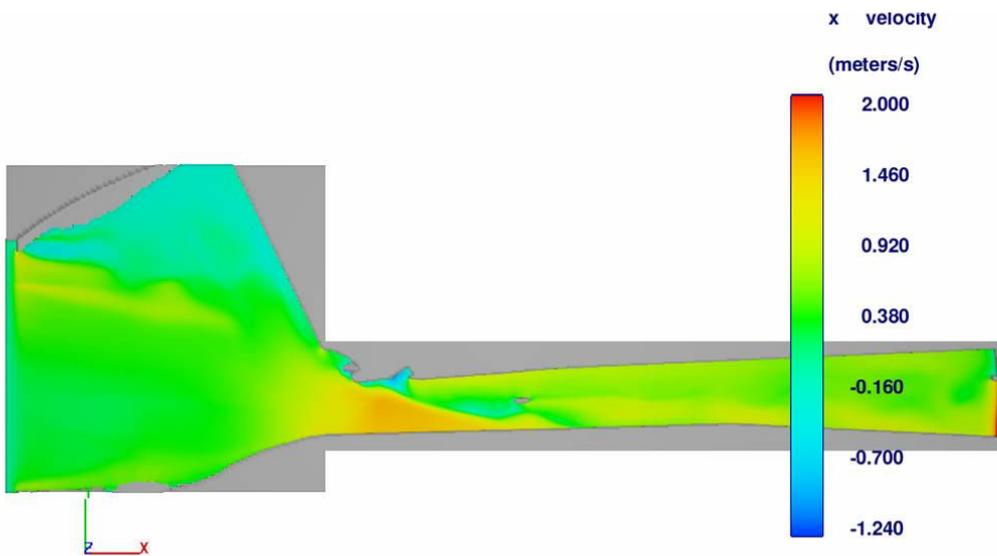
Fig. 7. Existing condition without pier at the flow  $Q_{S2} = 18.3 \text{ m}^3/\text{s}$
