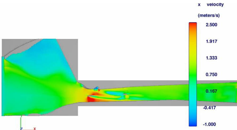
Fig. 8. Modification of the left wing wall of the intake at the flow  $Q_{S1+S2} = 24 \text{ m}^3/\text{s}$
