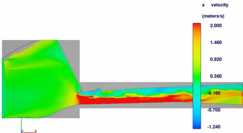
Fig. 5. Initial conditio of the intake at the flow  $Q_{S2} = 18.3 \text{ m}^3/\text{s}$
