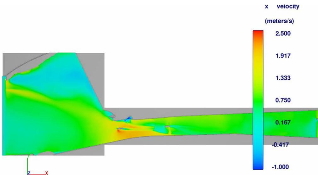
Fig.10. Widening of the right intake bank at the flow  $Q_{S1 + S2} = 24 \text{ m}^3/\text{s}$
