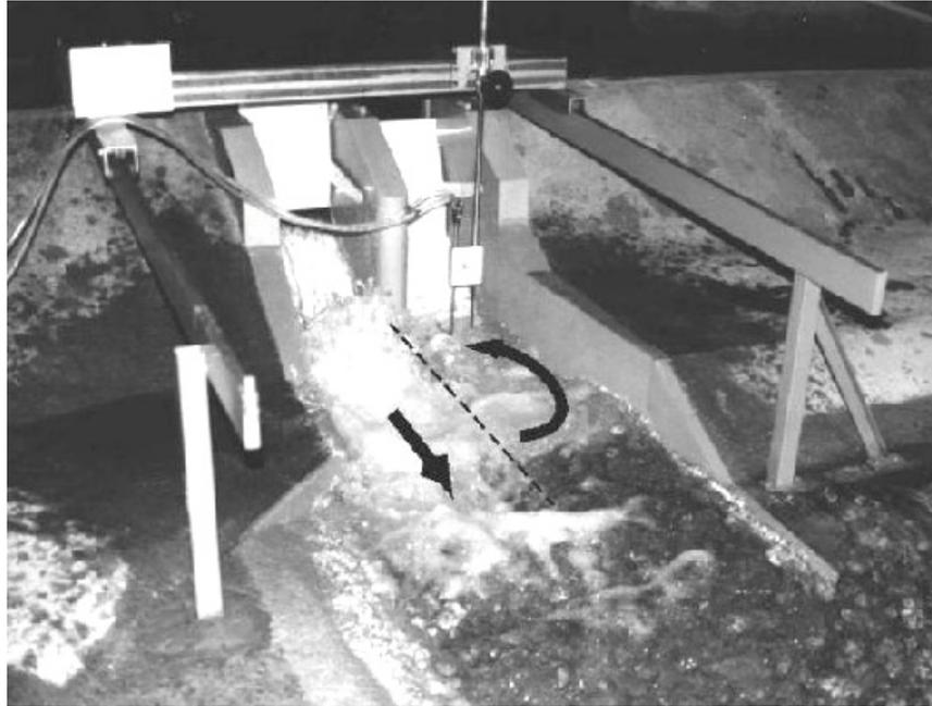
Fig 3: Original design – Flow over a single spillway section,  $Q=312 \text{ m}^3/\text{s}$  ,  $H_{TW} = 437.7 \text{ m a.s.l.}$  (regular tailwater level), gate opening  $a=4.0 \text{ m}$ ; The left margin of main flow and a dominant vortex in an inactive half of the stilling basin can be clearly seen.
