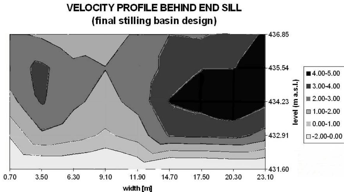
Fig 6: Final design –Velocity profile in cross-section immediately downstream of the end sill; Flow over a single spillway section,  $Q=312\text{ m}^3/\text{s}$ ,  $H_{TW} = 437.7\text{ m a.s.l.}$  (regular tail water level), gate opening  $a=4.0\text{ m}$ , right spillway in operation;
