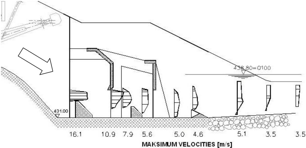
Fig 5: Intermediate design – Velocity profile changing alongside stilling basin
