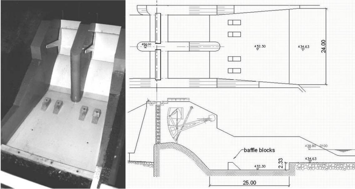
Fig. 1: Spillways and stilling basin of HPP Moste III – original design
