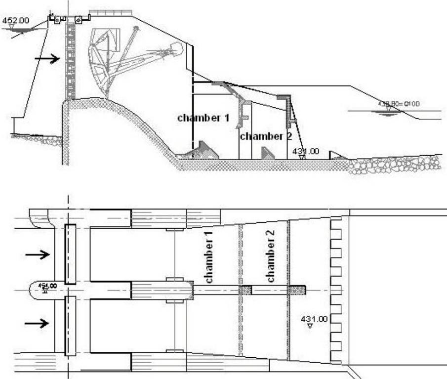
Fig 4: Final design – Stilling basin, equipped with dissipating elements
