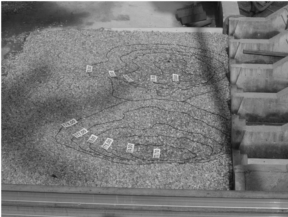
Figure 1: River bed mapping with wool threads
